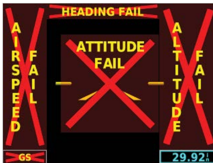
Figure 1-2 G5 PFD Page Failure Annunciations
