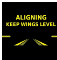
Figure 1-5 Attitude Aligned Keep Wings Level Indication
