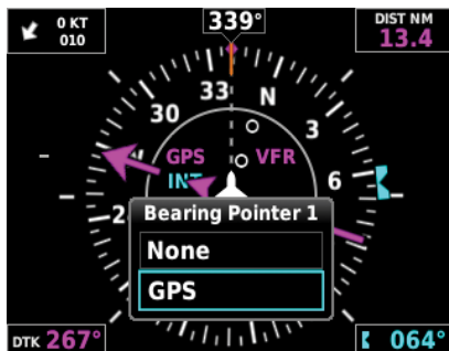
Figure 2-21 Bearing Pointer Source Options
