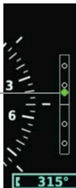
Figure 2-25 Vertical Deviation Indicator (Glideslope ILS Source) - HSI
