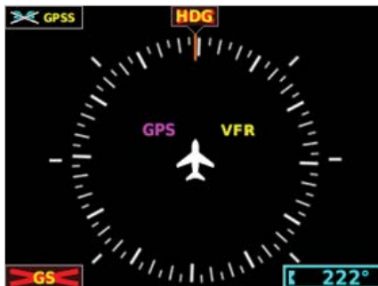
Figure 1-3 G5 HSI Page Failure Annunciations
