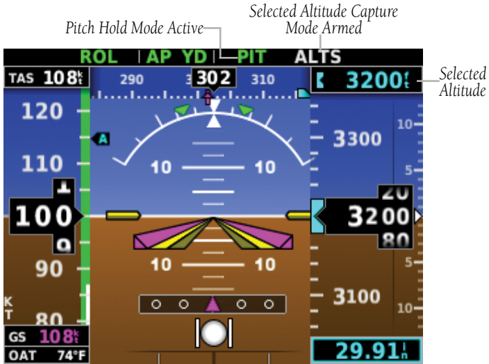
Figure 3-8 Pitch Hold & Selected Altitude Capture Modes
