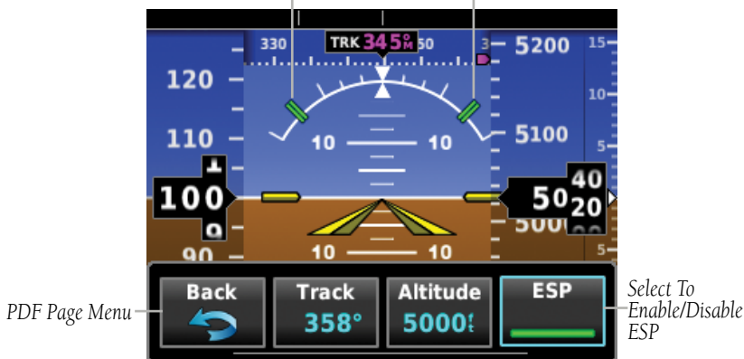
Figure 3-26 AFCS (ESP Enabled)
