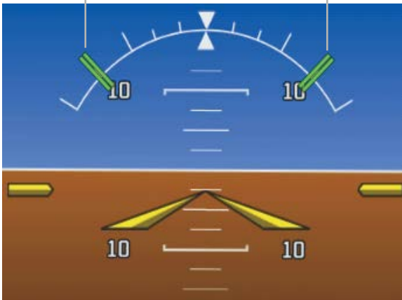
Figure 3-27 ESP Roll Engagement Indication (ESP Enabled but NOT Engaged)
