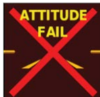
Figure 1-6 Attitude Failure Indication
