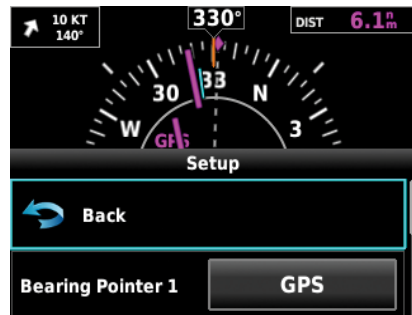
Figure 2-20 Bearing Pointer Setting
